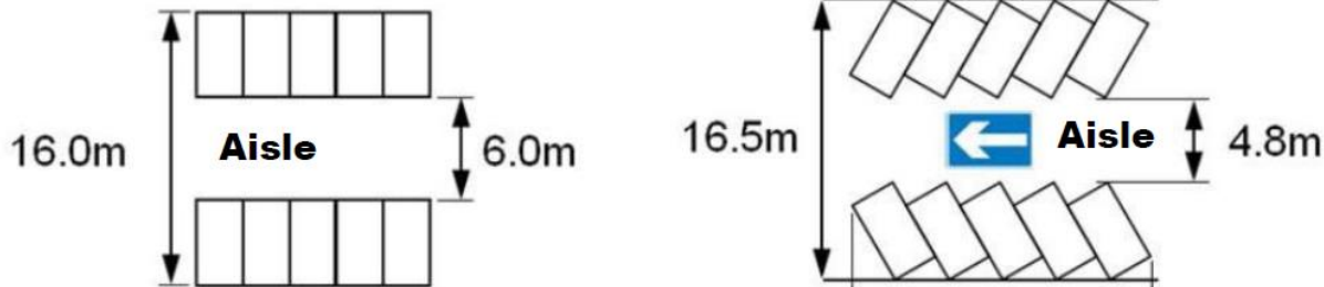
Figure 3.2: Examples of Parking Aisle
