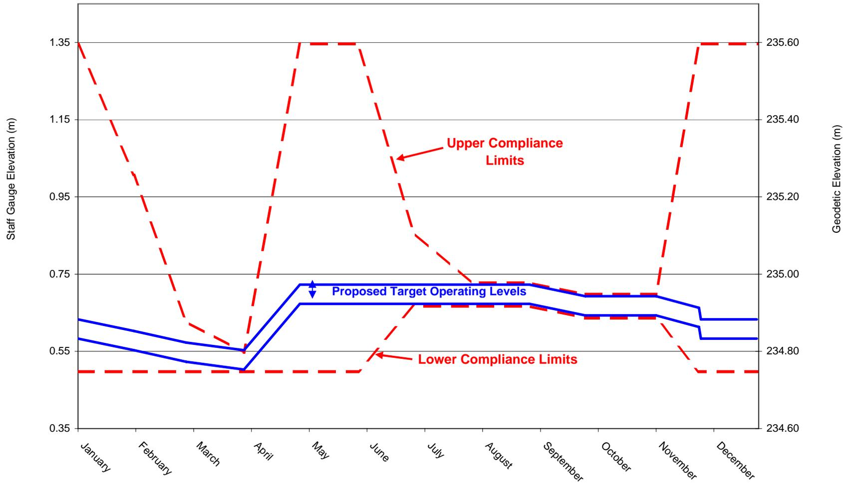
Fig. 10.2 Chiblow Lake Dam Operating Plan
