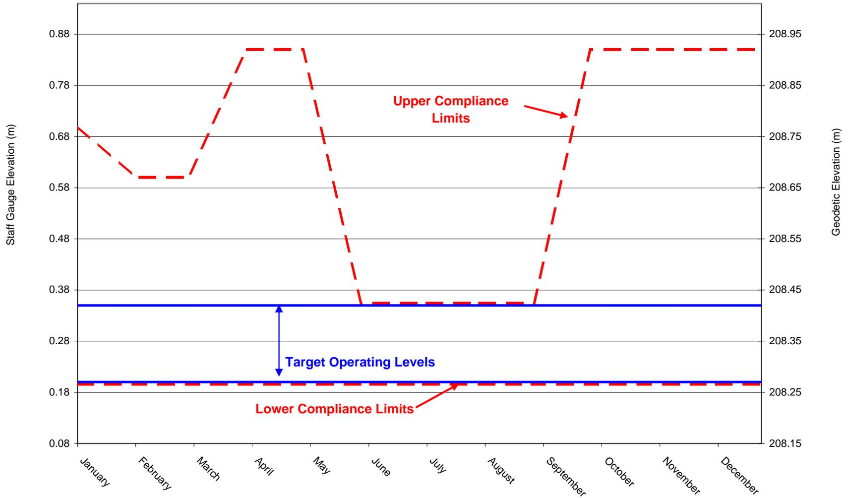
**Fig. 10.4 Blind River Dam Operating Plan**
